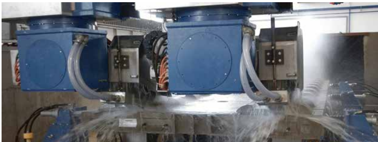
2 | Sanding machine sanding the cured rail track elements.
